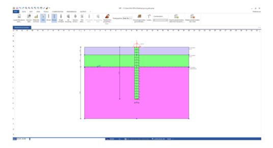
Pile and micropile software is intended for calculation of the bearing capacity of the foundation terrain of a pile or micropile in whatever load distribution (moment, normal force, shear).
