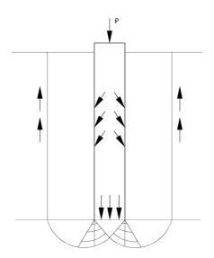
For soil with friction ( $\phi$ ) and cohesion (c), unit resistance  $Q_p$  at the point is given by the expression:
