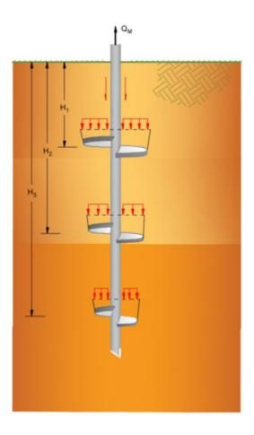
Development of Capacity for Multi-Helix Screw-Piles and Helical Anchors with S/D >3.
